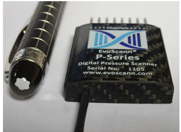
EvoScann® P-Series are highly-miniaturised pressure scanners designed specifically to meet the stringent demands of the aerodynamic testing industry where development is rapid and continuous. Utilising the latest in miniature scanner technology, P-Series is at the forefront of pressure measurement in challenging aerodynamic locations. The P-Series has been designed, from the start, with physical size, weight, accuracy and functionality in-mind and is available in a variety of configurations.
