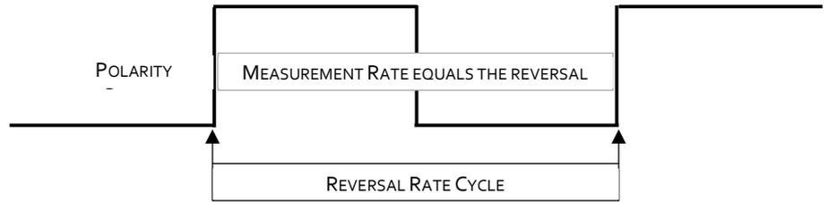
Like all of our new 664o Series Bridges, Guildline’s 664oQ QHR Bridge **decouples the polarity reversal rate** from the measurement rate allowing **measurements to be made much faster** than competitive DCC bridges. As shown in the right figure, you can independently specify a measurement rate and a reversal rate.
