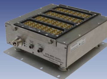
Intelligent 16, 32, and 64 Ch. Thermocouple Scanner
