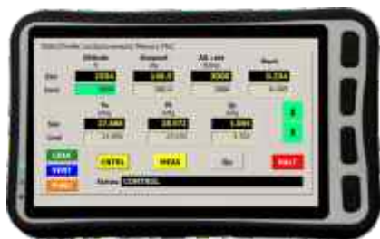
Optional MPSRW wireless remote terminal with backlit 7" LCD touchscreen
